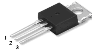
1. Gate 2. Drain 3. Source
