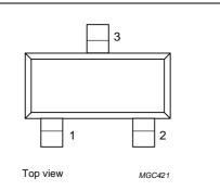
Fig.1 Simplified outline (SOT23) and pin configuration.
